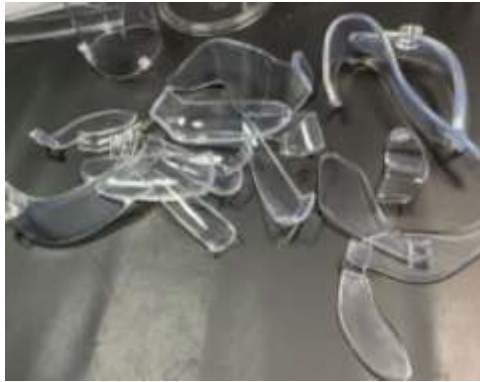
Figure 17: The wings are printed with transparent resin material Photo credit: Researchers
